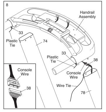
9. Set the handrail assembly on the Uprights (74, 78). **Be careful not to pinch the wires.**
